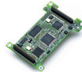
DSP Control Board
